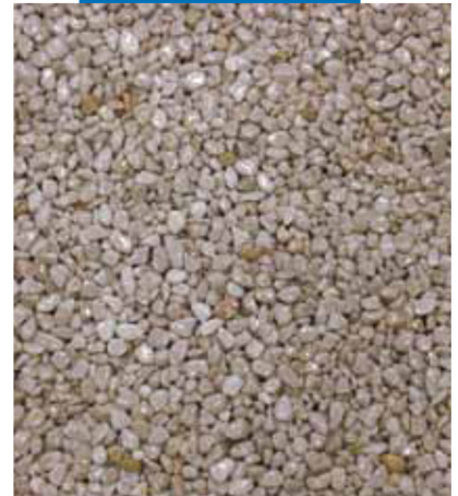
Application of the mixture of natural aggregates + Mapefloor I 910
